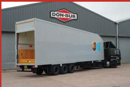
▲ Don-Bur's Blade™ panel can provide operators with a capacity of 52 GKN pallets on a standard 13.6m Lifting Deck trailer.
