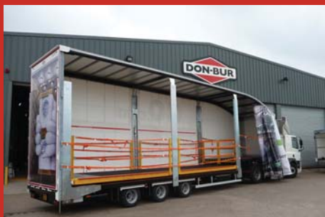
▲ 13.6m Curtainsided Lifting Deck
