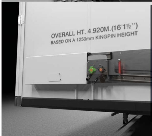
6) The lock handle can then be released. This prevents the coupling plate from moving.
