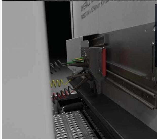
5) When coupling is complete, the operator should lift the lock handle into its upward position and push the coupling plate back into its stowed position.
