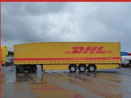
*LST solution with a fixed axle bogie.*
