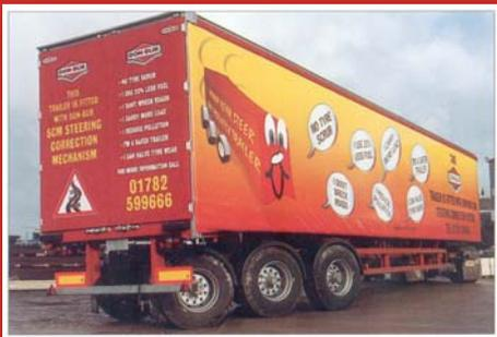
*2004: Don-Bur's first 16m long trailer with "SCM" active steering correction mechanism.*
