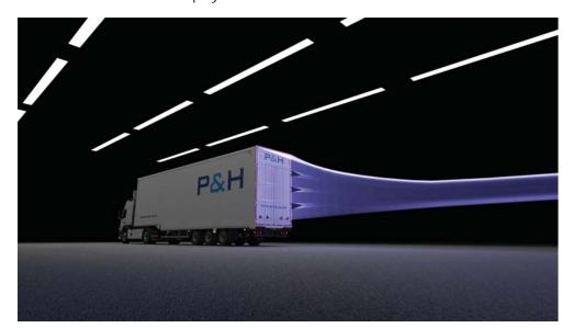
Studies on standard physical boat tails have found that up to 7% in fuel reduction can be achieved and plasma actuators are expected to generate similar fuel savings. However, many operators are unwilling to invest in standard physical boat tails due to the high risks of damage and associated costs to repair.
