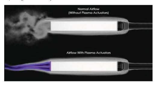
As part of Don-Bur's ongoing approach to providing aerodynamic, fuel saving solutions, further studies are ongoing to determine potential benefits as a result of positioning plasma actuators on additional areas of the trailer.
