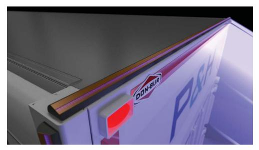
The Plasma Actuators are positioned at the end of the trailer along the sides and top of the rear frame and are angled inwards and downwards, respectively. Once activated, the resulting airflow is up to 10 m/s, then to avoid any discomfort to pedestrians, they are deactivated by a speed sensor once the vehicle reaches less than 10mph.
